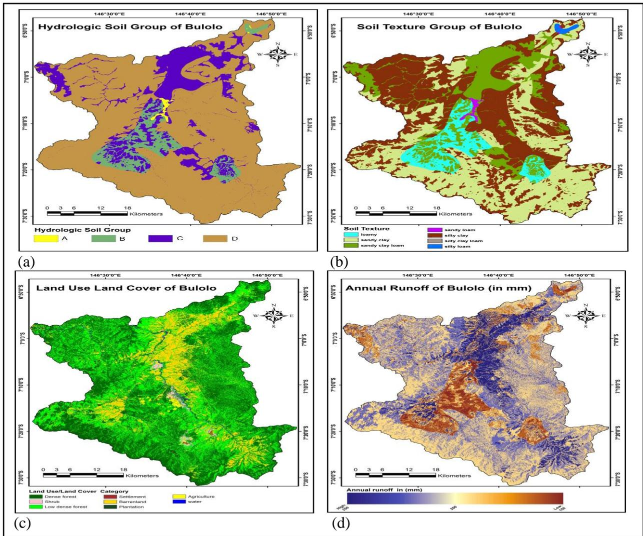
**Fig.6** Input maps for discharge. (a) Hydrologic Soil Group (b) Soil Texture Group (c) Land Use/Land Cover (d) Annual Runoff in mm.
