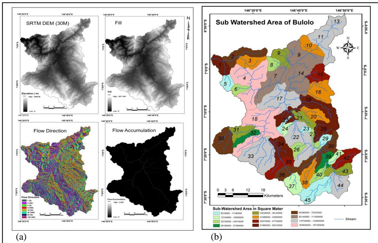
Fig. 4. Watershed Delineation:(a) Sub watershed delineation process (b) Sub watershed areas
