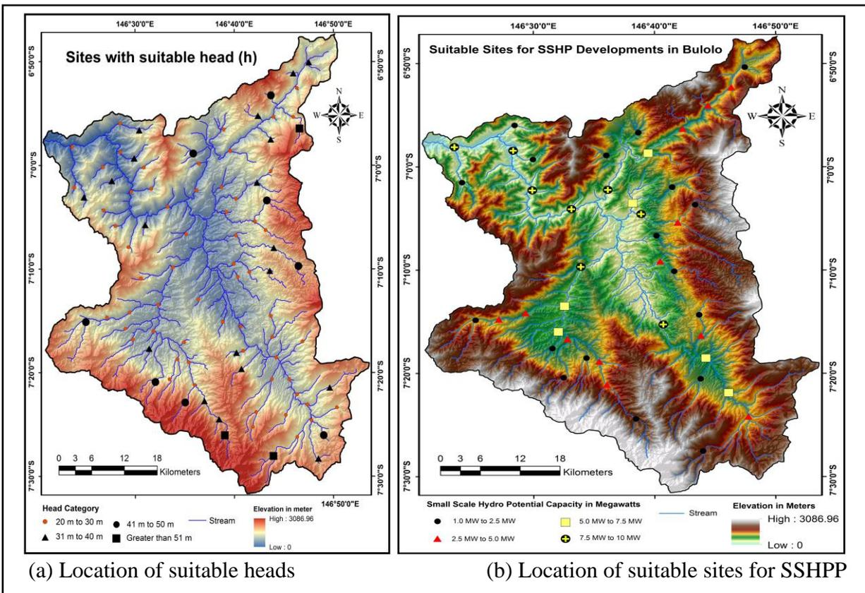
Fig. 7 (a) Location of suitable heads. (b) Location of suitable sites for SSHP
