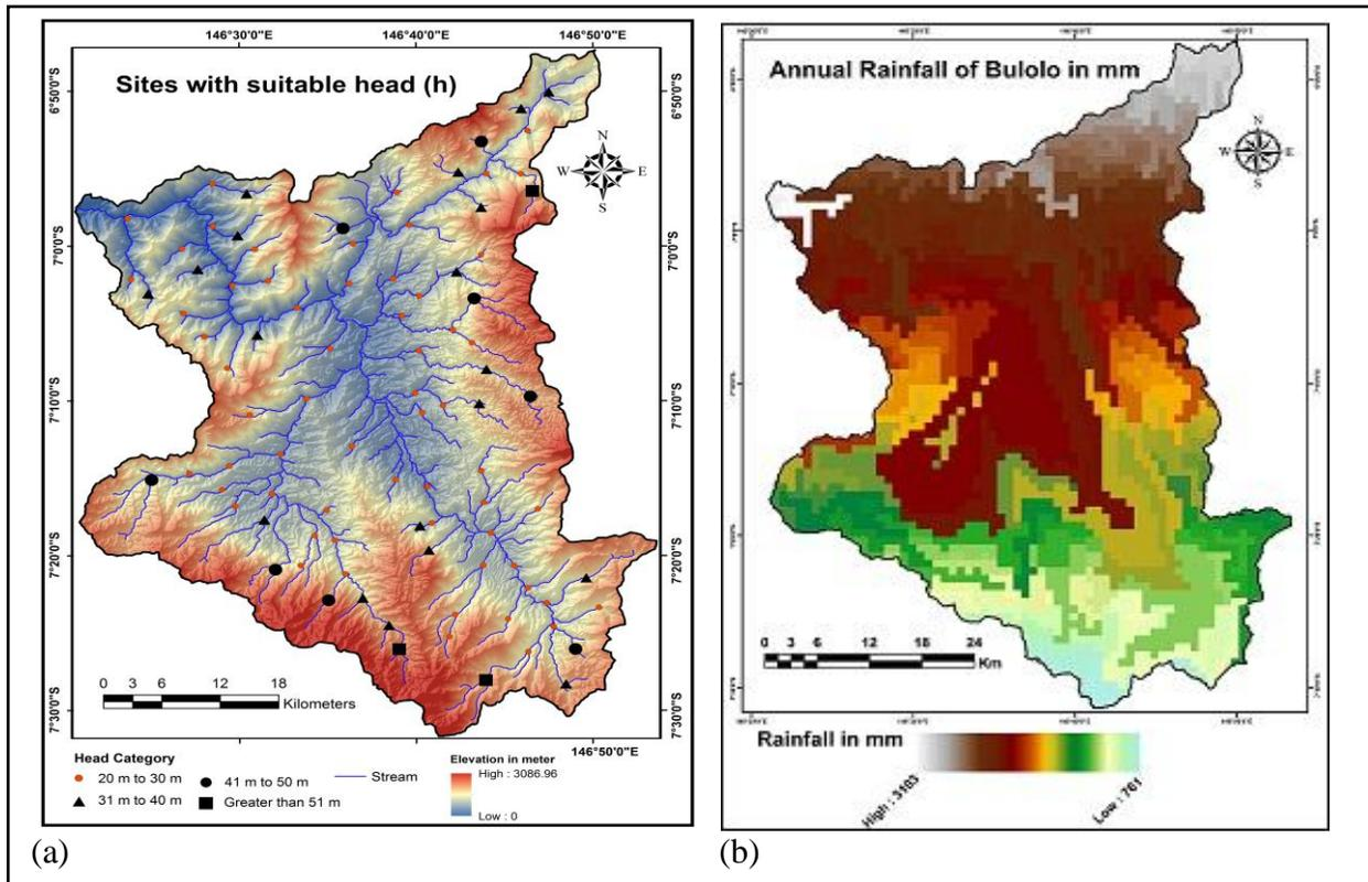
**Fig 5.** a. Sites with suitable heads, b. Annual rain fall in mm
